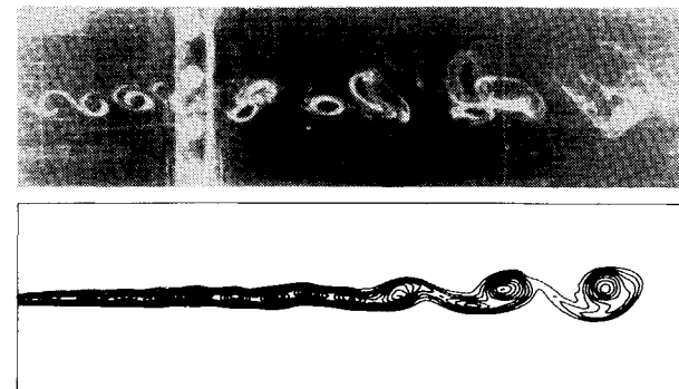
Fig. 7 Experimental flowfield and numerically generated vorticity contour plot for a mode III configuration.
